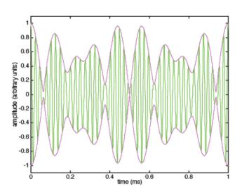
Next, the ideal envelope (square-rooted audio) for equal-amplitude 7kHz and 9kHz signals is shown on the same plot as the uncorrected SSB envelope:
