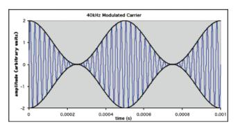
The envelope function in this case is  $E(t)=1+\cos(2^*\pi^*2kHz^*t)$ , or  $-[1+\cos(2^*\pi^*2kHz^*t)]$ . With an amplitude modulated carrier, the envelope is simply proportional to the modulation signal, plus an offset constant. Also notice that the lower envelope is a mirror image of the upper one.
