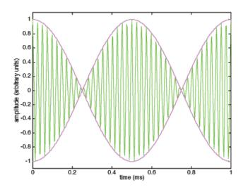
When this signal is squared by the process in the medium of air, you get back your original audio frequency of 2kHz, with zero distortion because no other frequencies are present. In other words, for a single-tone case, SSB gives a distortion-free signal with no pre-processing or additional signal conditioning.
