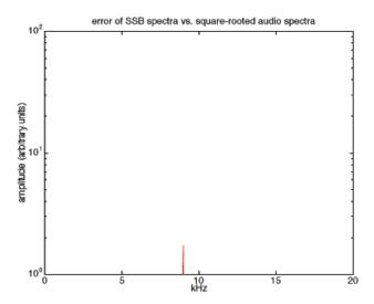
You can see that the 2kHz error term is gone, but a new one at 9kHz has appeared. However, the new error term is approximately 10dB lower in amplitude than the original 2kHz error term was.
