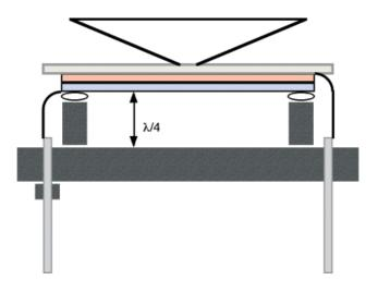
When a voltage is applied across the pins (that are protruding downward), the red element gets longer while the blue one shortens, causing a bend in the bimorph. When the polarity changes, the opposite bend occurs. The maximum displacement change is in the center of the element where the cone is attached. This way, the cone undergoes maximum displacements. Also, the outer edge of the cone moves as much as three times further than the inner portion as it flexes.
