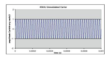
The black line running across the peaks of the wave is the envelope. Notice there is also a black line running across the troughs. This can also be used as the envelope boundary. As a rule, the lower envelope is a mirror image of the upper one. Below is the same 40kHz carrier, now being amplitude modulated by a 2kHz tone.
