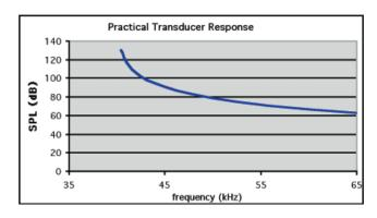
As you can see, this is much more realistic. Because the upper sideband levels are so much higher, the overall performance will be much better. In fact, the output levels will be increased by more than 56dB over the band of concern. Such an emitter is realizable. Also remember that there will be output below 500Hz, just not at the same level as the rest of the bandwidth.
