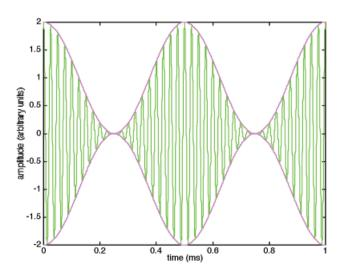
When this envelope is squared by the process in the medium of air, the 2nd harmonic ends up with the same amplitude as the fundamental or 100% THD as was mentioned earlier in the paper.
