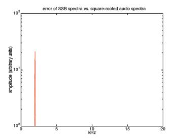
You can see that the only error term is at 2kHz. It can be proven mathematically that the only error term that results in the SSB envelope is in fact the 2kHz signal shown. However, if a 2kHz "correction term" (with the proper phase and amplitude) is injected into the modulator, the unwanted 2kHz error term can be suppressed completely.
