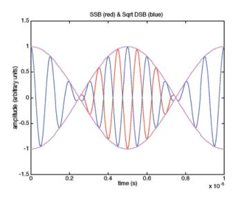
The blue DSB line lies on top of the red line when their values are the same, so when only the blue line can be seen, the red trace is underneath it. Both of these methods give the same envelope that will demodulate into a single, distortion-free audio signal (in this case, 2kHz). However, the spectrums required to generate these two envelopes are vastly different. Lets look at them. Here is the SSB spectrum with two frequencies:
